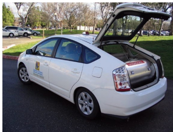
Cryo-Compressed Vessel Installed Onboard the Prius Hydrogen-Fueled Hybrid Vehicle
