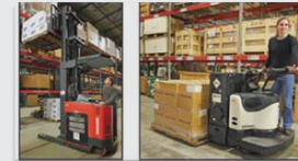
Class-1, -2, and -3 Forklifts Plug Power (GenDrive FCs)
